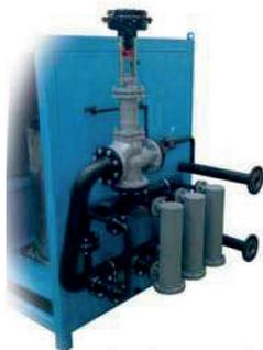
3 channel valve on cooling circuit
